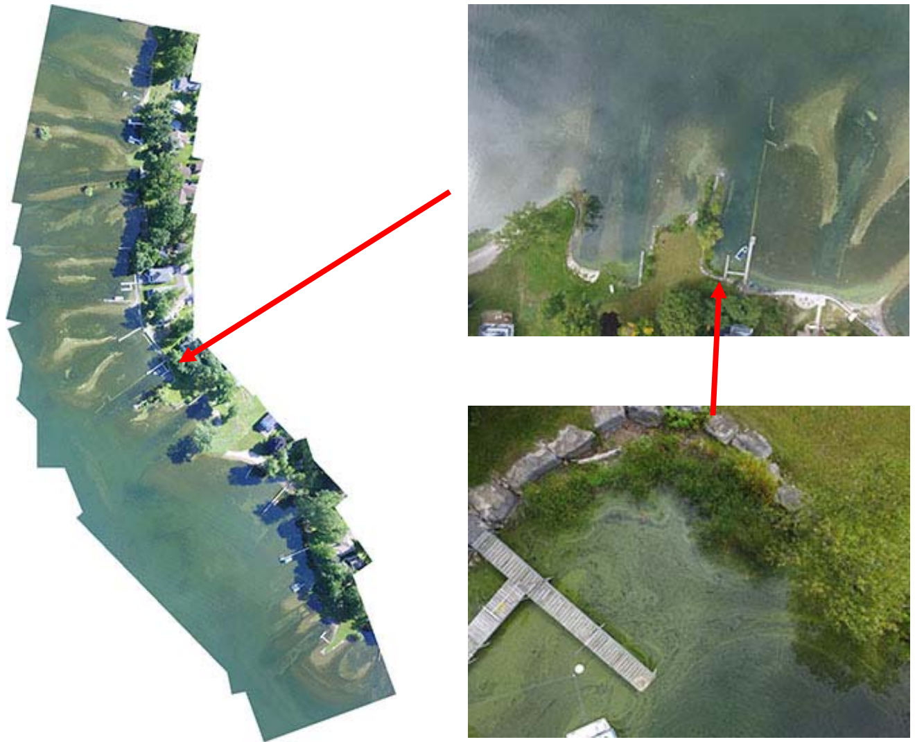
Fig. 10. Spliced drone images from Burtis Pt on 6/18 (left), Burtis Pt from 100m altitude on 9/23 (top right) and Burtis Pt from 25 m altitude (bottom right). The BGA blooms are barely visible at 100 m but are visible from 25 m.
